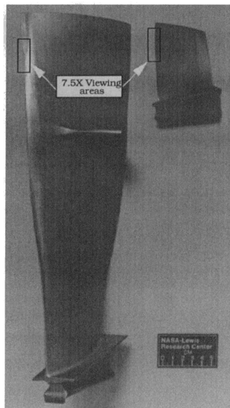
Fig. 1(a) Comparison between engine fan blade and the research rotor blade
